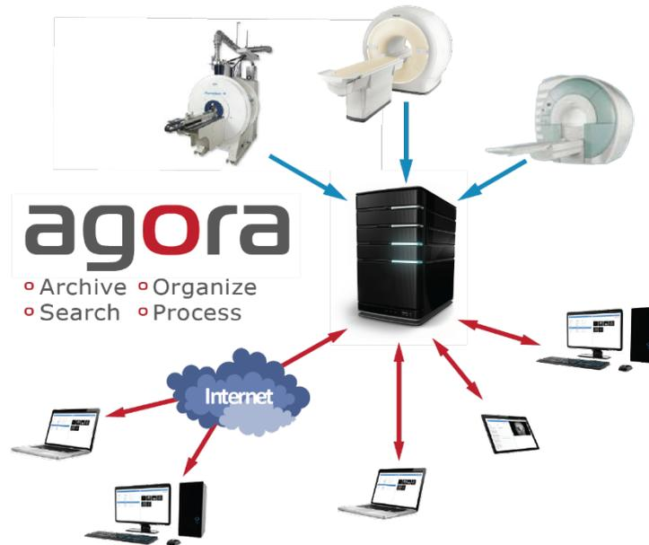
With Agora, you can easily configure an environment that exactly matches the needs of your lab for data organization and accessibility. Connect multiple scanners that will automatically feed raw-, image-, and meta-data to the Agora platform. Your data remains in-house and you can implement or use your own existing data backup solutions. Users access data selectively using a web browser and a personalized account.
